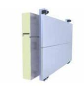
To accommodate thermal movement, the modular click rail SE is supplied pre-punched with alternative round and slotted holes. One fixed point is required per rail. The optimal configuration is to make the fixed point in the same position in each rail.
