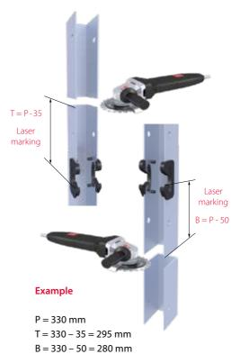
Insert the adapter into the modular click rail. For the upper adapter check the distance between the lower edges of adjacent inlays is equal to the transition panel cover width, P.
