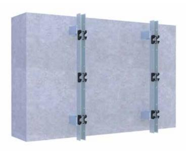
**Fixed point**Rivets or screws fixed in circular holes (on **both** sides of the U-
