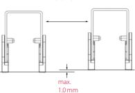
3. Vertically adjacent modular click rails must be aligned within 1.0 mm of each other.
