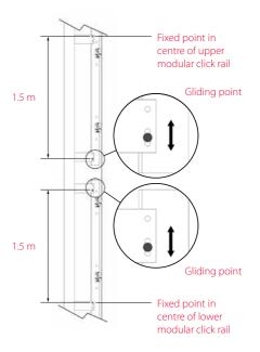
To make the sliding point effective, a spacer pad must be used with the rivet gun to ensure the rail is free to expand and contract.
