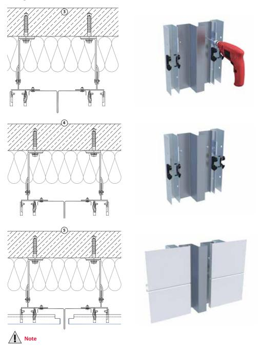
The flashing support should never be used to fix modular click rails to the sub-construction.
