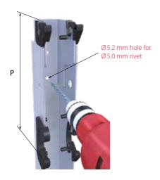
For the lower adapter, check the distance between the upper edges of adjacent inlays.
