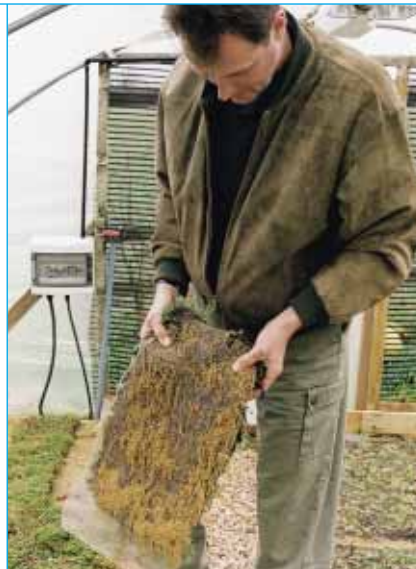
Examining sedum mat root structure
